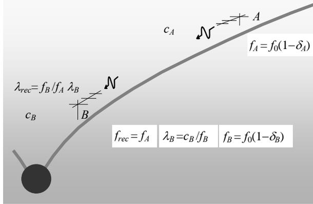
Figure 3.2.3-1. The velocity of light is lower close to a mass center,  $c_B < c_A$ , which results in a decrease of the wavelength of electromagnetic radiation transmitted from  $A$  to  $B$ . Accordingly, the signal received at  $B$  is blueshifted relative to the reference wavelength observed in radiation emitted by a similar object in the  $\delta_B$ -state. The frequency of the radiation is unchanged during the transmission.
