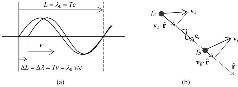
Figure 3.2.4-1. (a) The wavelength of electromagnetic radiation emitted by a moving source is shortened in the direction of the motion by the distance moved by the source during the cycle time,  $\Delta\lambda = \lambda_0 v/c$ . (b) The Doppler effect combines the effects of the velocities of the source and the receiver in the direction of the signal path.
