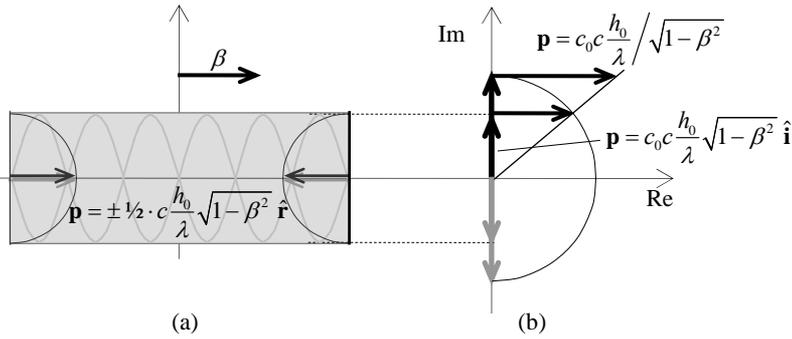
Figure 2.2.2-1. An electromagnetic resonator can be studied as an energy object or closed energy system with rest mass equal to the sum of the mass equivalences of the waves in opposite directions.
