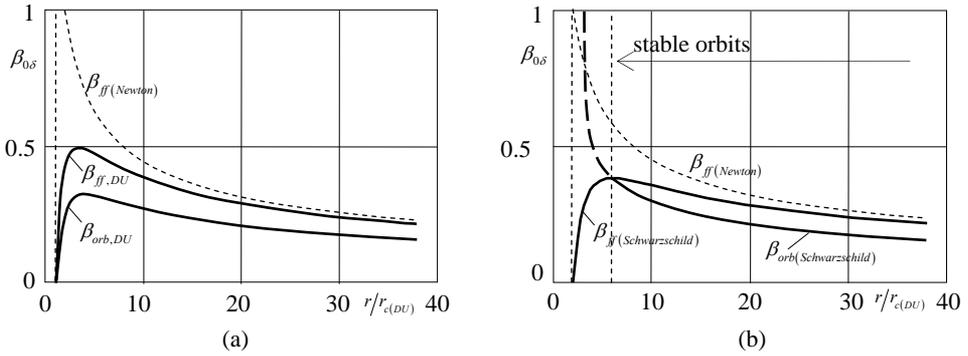
Figure 3.1.2-1. The velocity of free fall and the orbital velocity at circular orbits: (a) in DU space, (b) in Schwarzschild space. The velocity of free fall in Newtonian space is given as a reference.
