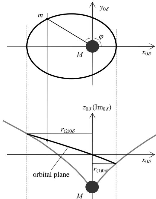
Figure 3.1.1-2. Projections of an elliptic orbit on the  $x_{0\delta}$ - $y_{0\delta}$  and  $x_{0\delta}$ - $z_{0\delta}$  planes in a gravitational frame around mass center  $M$ .
