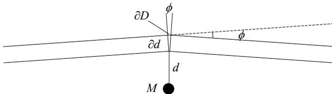
Figure 3.2.2-1. Light ray passing a mass center in space is bent due to a reduced velocity and increased distance close to a mass center.
