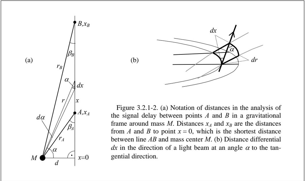
Figure 3.2.1-2. (a) Notation of distances in the analysis of the signal delay between points  $A$  and  $B$  in a gravitational frame around mass  $M$ . Distances  $x_A$  and  $x_B$  are the distances from  $A$  and  $B$  to point  $x = 0$ , which is the shortest distance between line  $AB$  and mass center  $M$ . (b) Distance differential  $dx$  in the direction of a light beam at an angle  $\alpha$  to the tangential direction.
