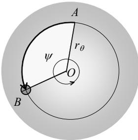
Figure 3.2.5-2. Clock transportation by longitudinal angle  $\psi$  from point  $A$  to  $B$  at latitude  $\theta$ . The delay due to the additional (slow) velocity is mathematically identical to the Sagnac delay of light transmission from point  $A$  to  $B$  (through links following the surface of the Earth at the same latitude).
